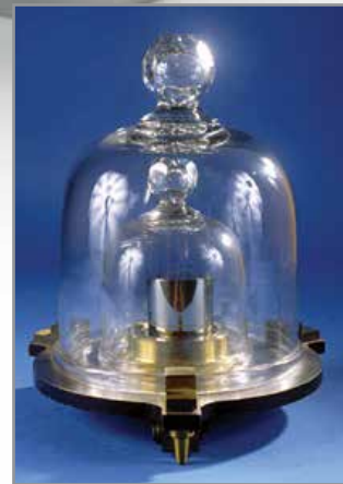
Up until the SI redefinition in 2019, the National Institute of Standards and Technology (NIST) housed and maintained America's official mass standards. Pictured above, the K20 kilogram mass standard served as the primary prototype national standard.
