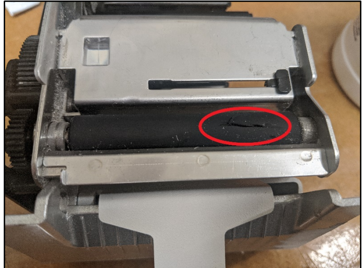
Figure 6 – Black rubber roller with damage
