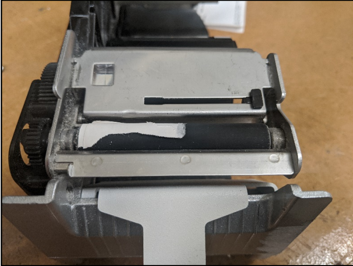
Figure 5 – Label debris stuck to black rubber roller
