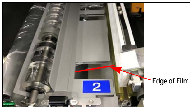
Figure 3. Film Out of Position
