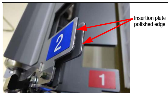
Figure 10. Insertion Plate Front Edge
