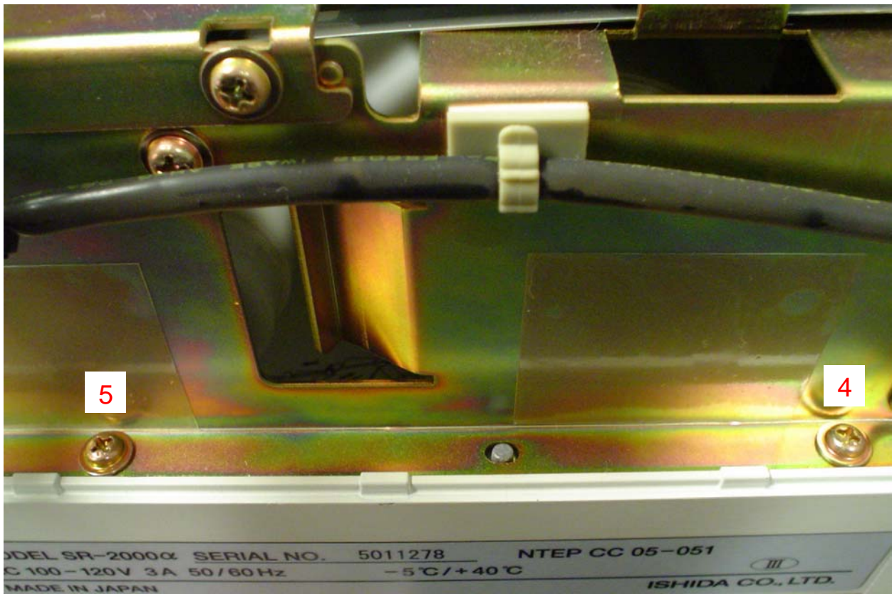
Figure 2. Locations of the two right-side frame screws (side view)
