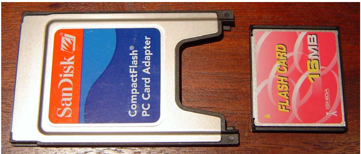
Figure 2. PCMCIA Compact Flash Adapter and CF Card
