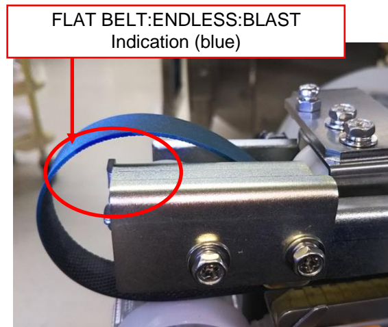
FLAT BELT:ENDLESS:BLAST installation image
