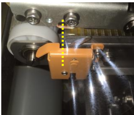
Even is the machine status is normal the film stop position varies approx. \pm 1 cm.
