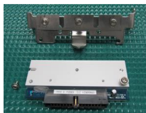
5) Remove thermal head by loosening the two screws indicated in the circles in the picture. Replace it with a new thermal head. To attach the thermal head, perform the procedure in the reverse order of detaching.
