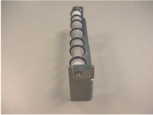
Check after attaching the standby roller
