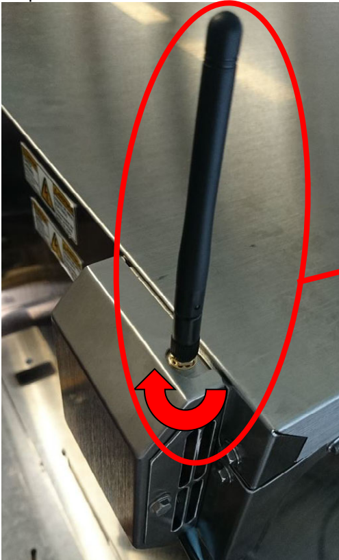
Step 12. Mount the Wi-PORT antenna.
