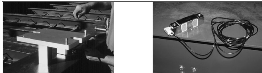
Figure 4-2. Baseplate and Load Cell
