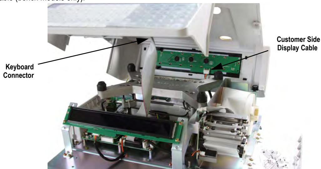
Figure 3-8. Unplug Cables from Top Cover
