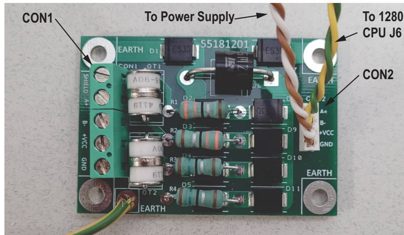
Figure 2-3. Wiring to RS-485/Power Supply Card
