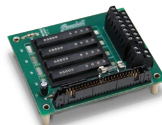
8-channel relay rack
